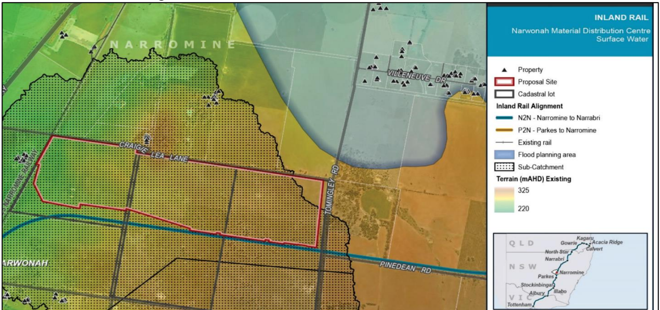
Figure 12: Narwonah Material Distribution Centre – Surface Water Source: ARTC In Land Rail – Review of Environmental Factors
